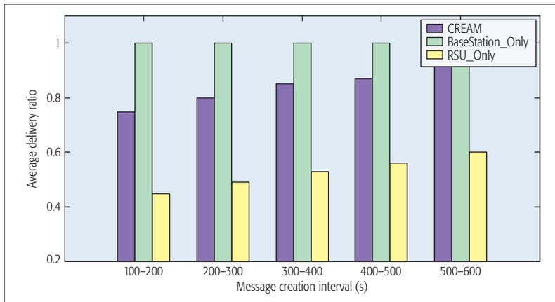
Figure 4. The performance of average delivery ratio.
