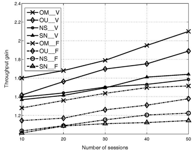
Fig. 4. Network throughput gain in the random topology.
