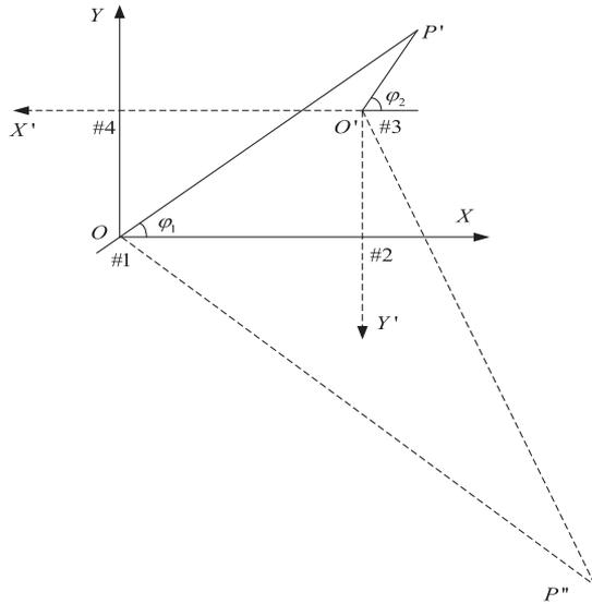
Fig. 2. Planar diagram of sensor array and azimuth of PD source.
