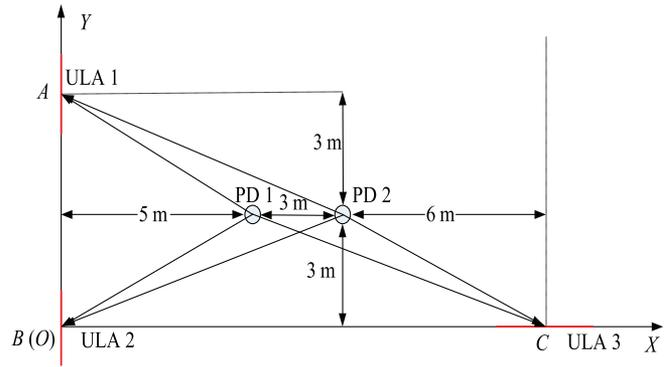
Fig. 9. Planar diagram of three ULAs and two PD sources.
