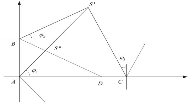
Fig. 3. Position of three ULAs and the actual and fake PD sources.
