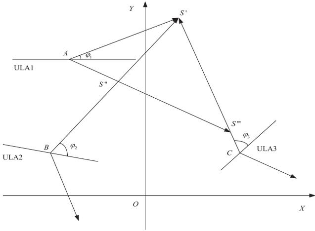
Fig. 1. Position of three ULAs and azimuth of PD source.
